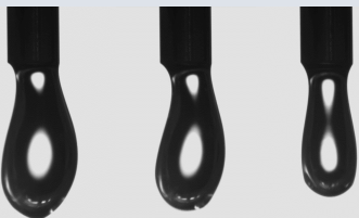
Figure 1. Snapshots of a video showing the remarkable viscoelastic behavior of a film at the solution/air interface of {4.1 mM C_{12}SO_4^- + 10 mM \alpha -CD + water} ( r = 0.41 ) at 283 K during drop volume reduction. Notice that there is no neck reduction.
